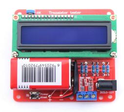
After all the installation, connect the power. Push the button, and maybe the screen will light without any character display. Don't be panic, right adjust the resistance and you will see the character.
